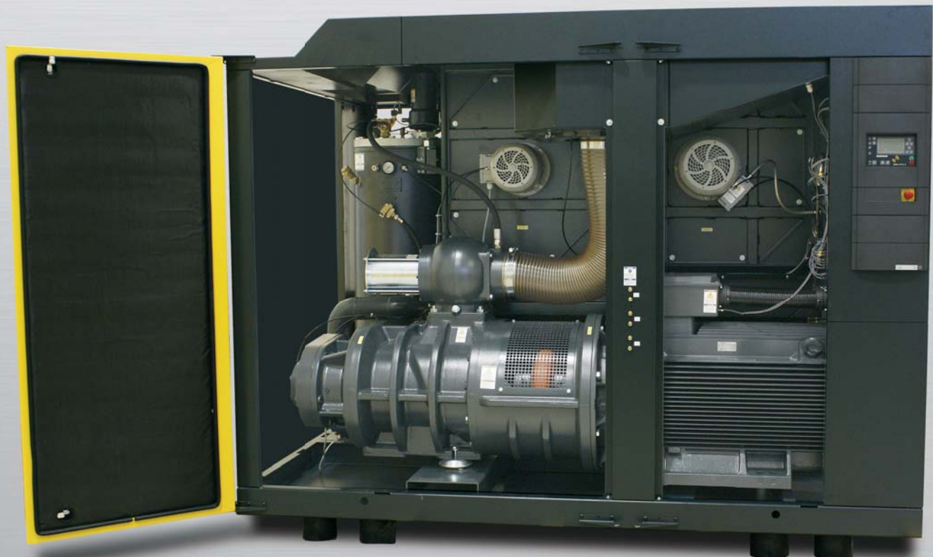
One-to-One Direct Drive Airend RPM = Motor RPM
